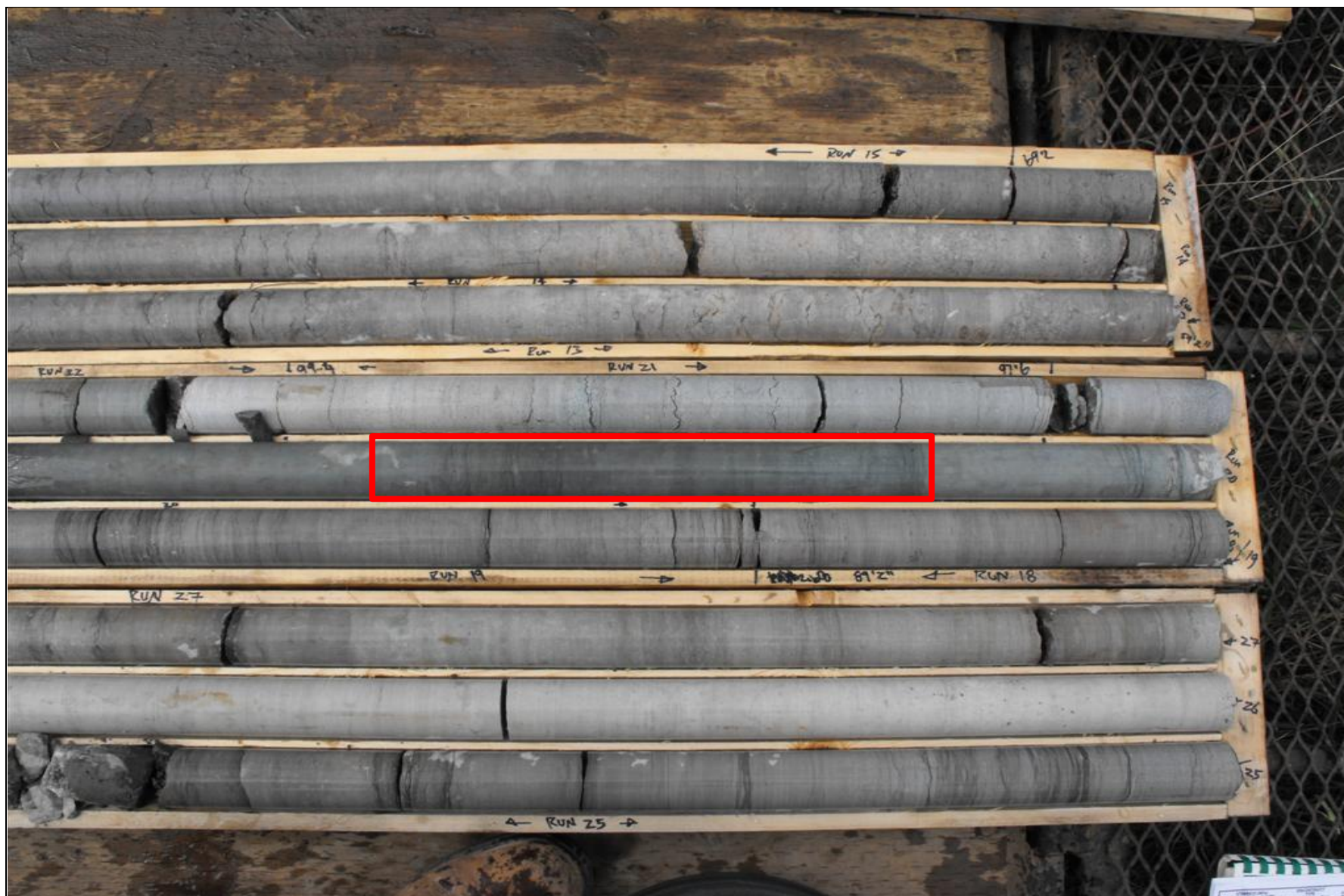
Photograph 1.1: Approximate Location of Upper Green Marker Bed – BH1-11
