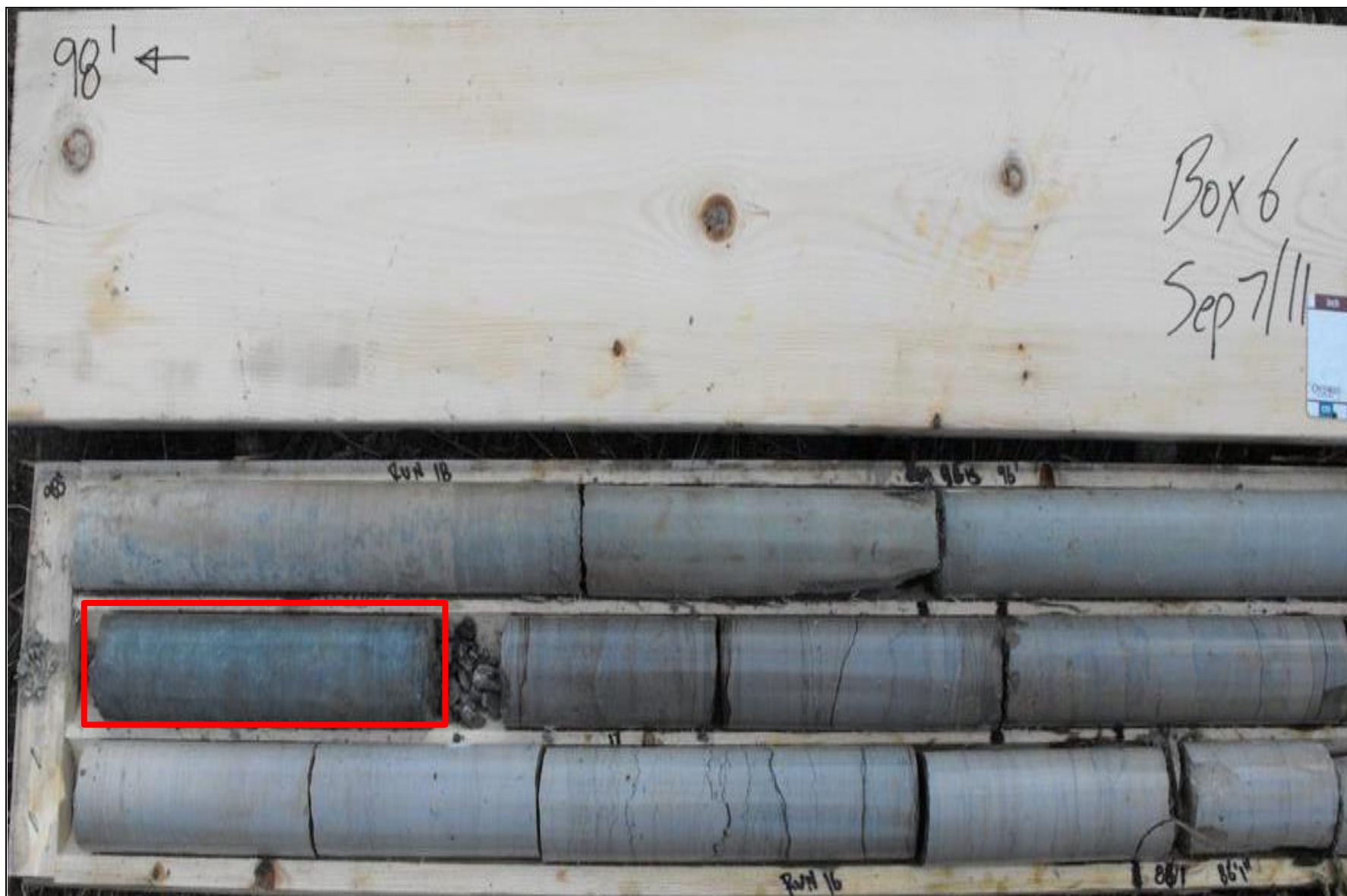
Photograph 2.1: Approximate Location of Upper Green Marker Bed – BH2-11
